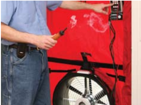
A blower door measures home air leakage
