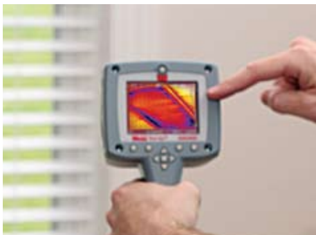
An infrared camera reveals hidden air leaks and inadequate insulation
